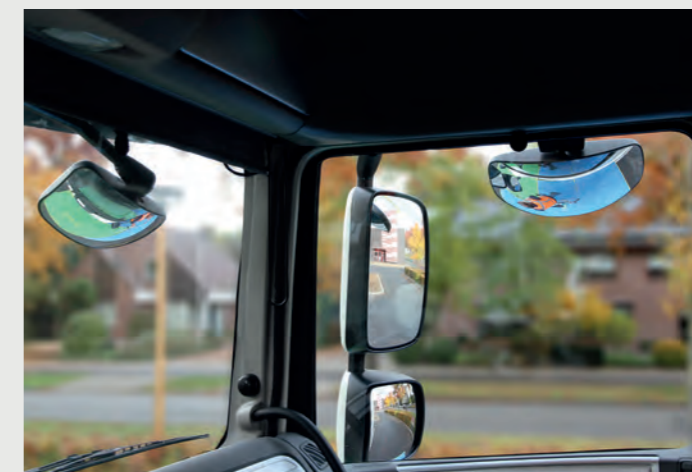
Truck with Front Mirror and Close-Proximity Mirror Although trucks are fitted with a front mirror and a close-proximity mirror, which cover the area in front of and to the right of the truck, there are still blind spots in this area.
