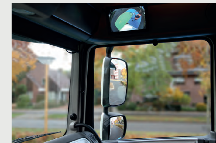
Truck with CornerEye (0400040) CornerEye replaces the front mirror and close-proximity mirror and offers an excellent view of the areas they cover and beyond with a single glance.
